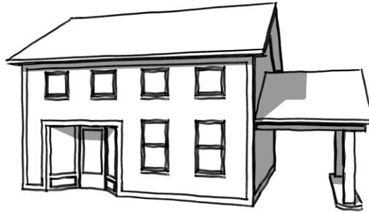
Figure 5. Drive-thru Businesses - Drive through businesses must have drive through facilities located to the side or rear of the building and the canopies shall relate in architectural style and design to the buildings to which they are attached.
