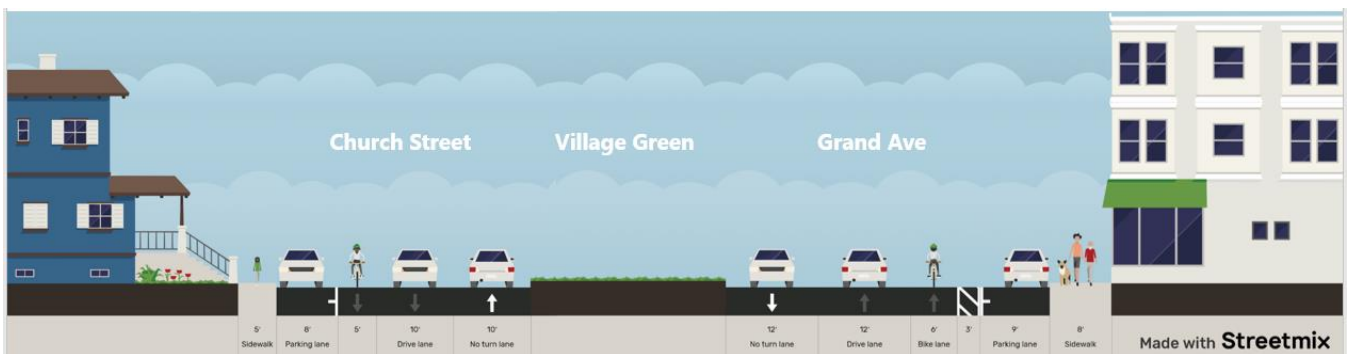
Figure 18. Cross Section View Looking North of Grand Avenue and Church Street for Alternative 2.
