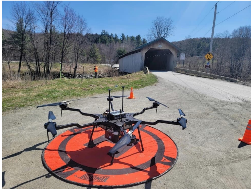
Figure 1. Topobathymetric LiDAR enabled UAS at the Longley Covered Bridge.
